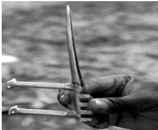
Air terminal for highest branches
